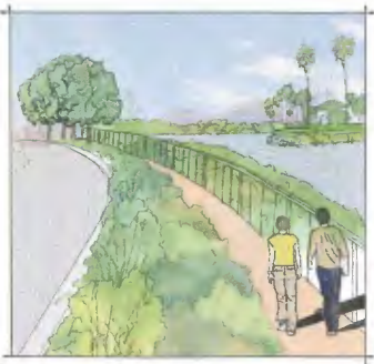
Admiralty Way: Parkway planting and path elevation change buffers pedestrian path from traffic.
